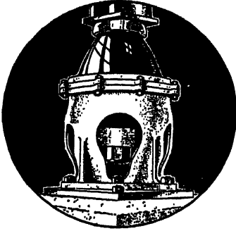
Porcelain insulator at the foot of a steel transmitting antenna tower.
